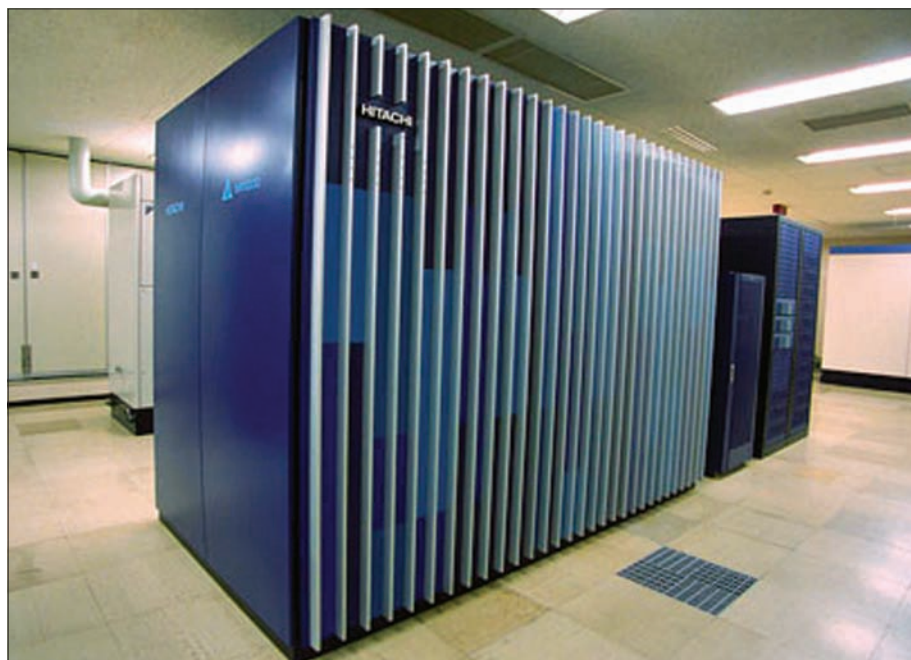
The Hitachi SR11000 model K1 supercomputer calculated the interior structure of a black hole. It provides a peak performance of 2.15 teraflops peak. (Courtesy KEK.)
